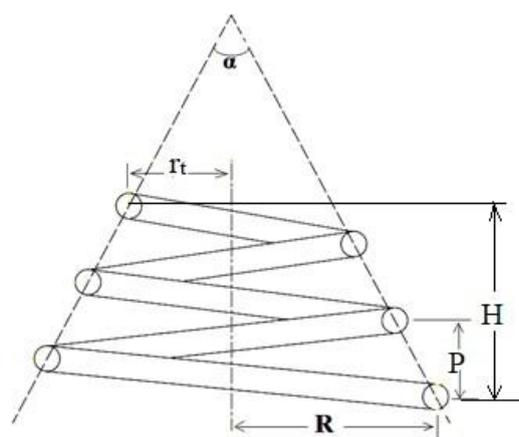
Figure 4.1 Basic geometry of a conical coil pipe
