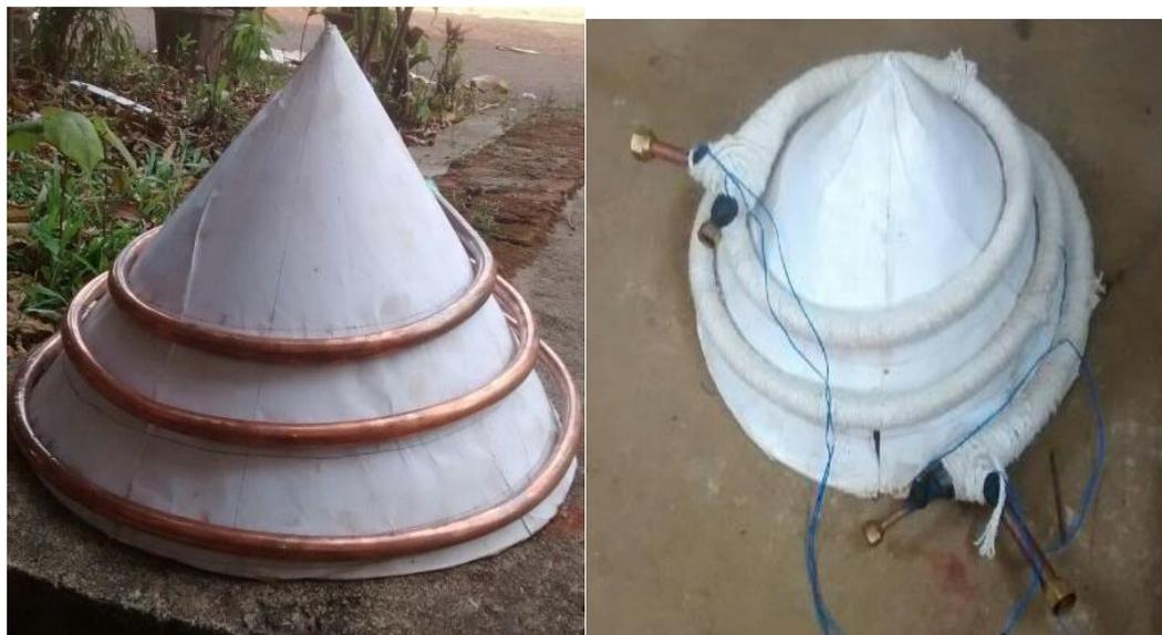
Figure 4.4 Fabrication of conical coil heat exchanger
