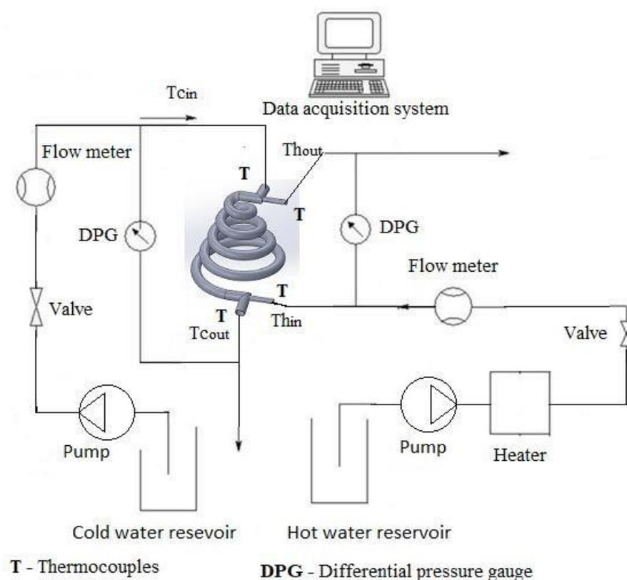
Figure 4.3 Experimental setup
