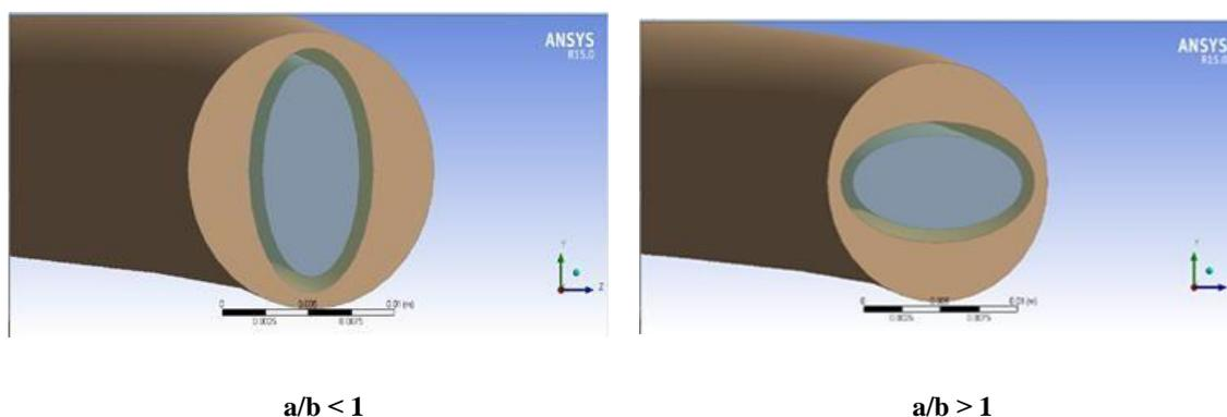
Figure 4.6 Configurations of the inner elliptical tube inside the circular tube
