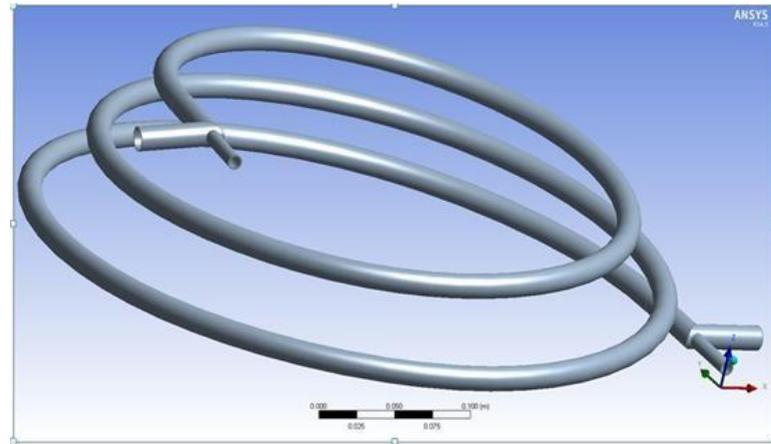
(a) Model of the conical coil heat exchanger
